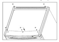
Check that the door is aligned vertically and horizontally to ensure proper opening and closing of the door.
